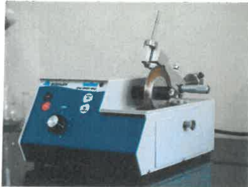
Figure 5. Buehler IsoMet low speed saw
