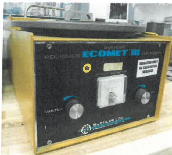
Figure 6. Buehler Ecomet III polisher and grinder
